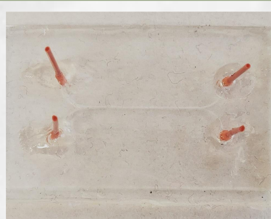
Replica Moulding with PDMS with connectors
