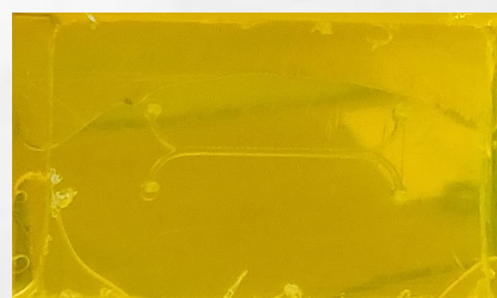
Replica Moulding with PDMS with connectors
