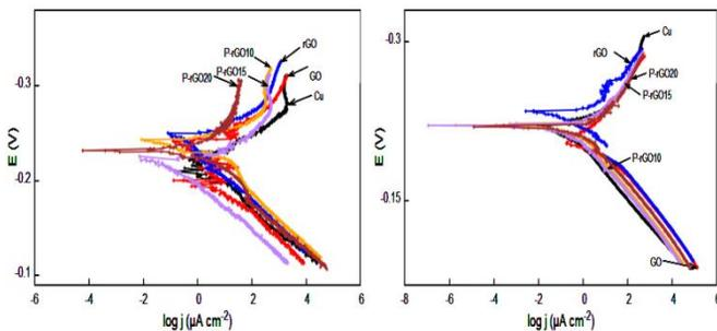
Fig. 4 Polarization curves for bare copper and coatings: measured directly after EPD (left) and after 10 days immersion in 3.5% NaCl solution (right).
