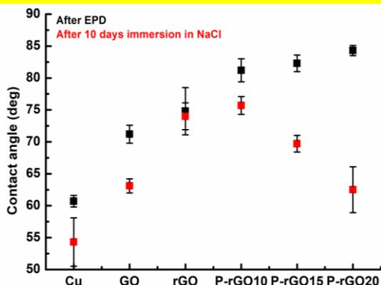
Fig. 3 Contact angle values for coatings: directly after EPD and after 10 days immersion in NaCl.
