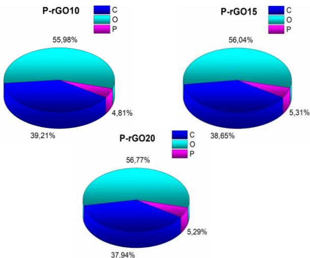
Fig. 2 Chemical composition of phosphorus functionalized reduced graphene oxide samples.
