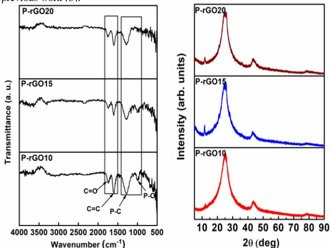
Fig. 1 FTIR spectra (left) and XRD patterns (right) for phosphorus functionalized reduced graphene oxide samples.
