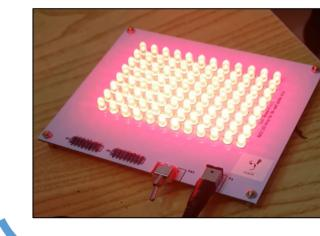
RED-LED array (light source with excitation wavelength: 640 nm, and voltage: 15 volt) composed of 96 LEDs in a 12 × 8 arrangement.
