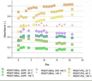
The graph shows that pristine PEDOT:DBSA possesses better long-term stability than pristine as well as heated PEDOT:PSS. Moreover, it can be further improved by cross-linking with GOPS, showing significantly reduced dissolution.
